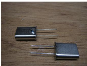
I make a small solder point on the good crystal on the pin edge and in the center and tin the lead end of the donor crystal...
