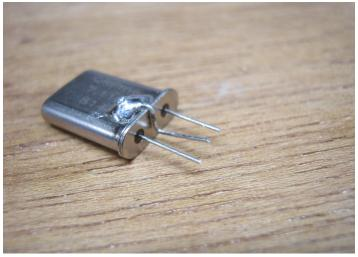
Then fold it over and out to make a phantom center pin and cut all 3 leads even with eack other.
